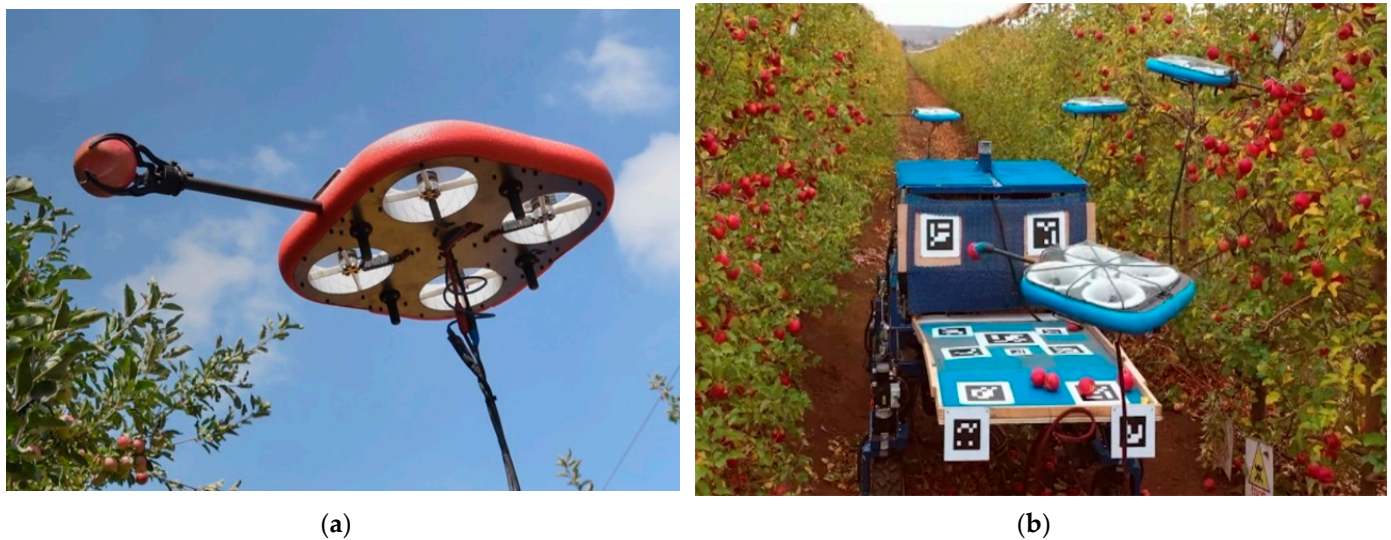
Figure 9. Telev aerial harvesting system: (a) flying autonomous robot (FAV); (b) wheeled base vehicle and four FAVs [88].
