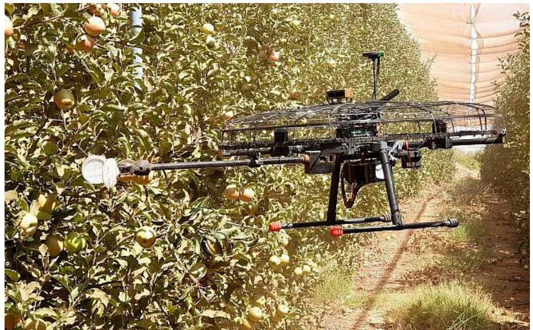
Figure 8. Tevel aerial harvesting robot; first prototype [88].
