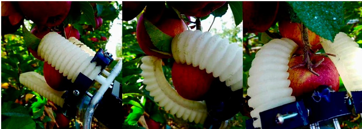
Figure 6. Indicative apple harvesting end effectors proposed by Hohimer et al. (Reprinted/adapted with permission from Ref. [63]. 2019, Hohimer, C.J.).
